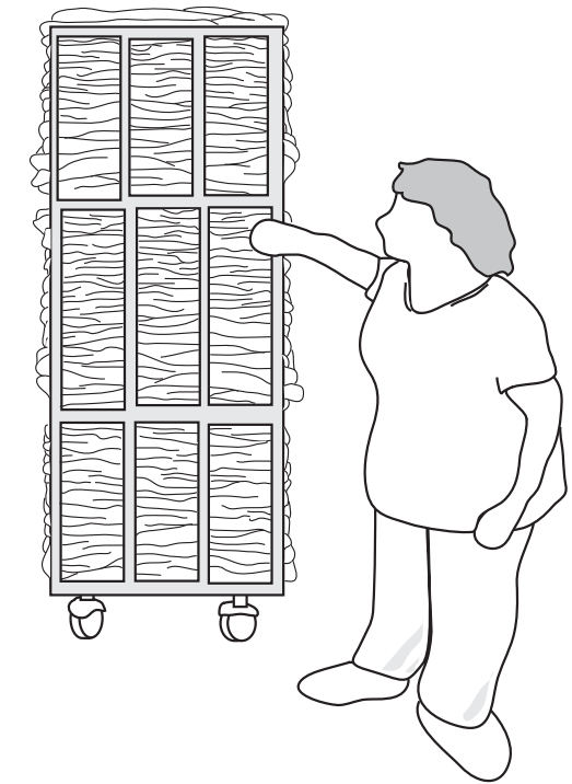
Figure 2.1 Leading a cart by pulling with one arm can place the shoulder in an awkward posture.
