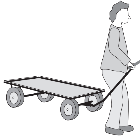
Figure 4.5 T-bar handles are an appropriate choice for carts that need to be pulled.
