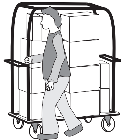
Figure 4.6 Carts with vertical poles are useful when the load is high enough to obstruct visibility from the back.
